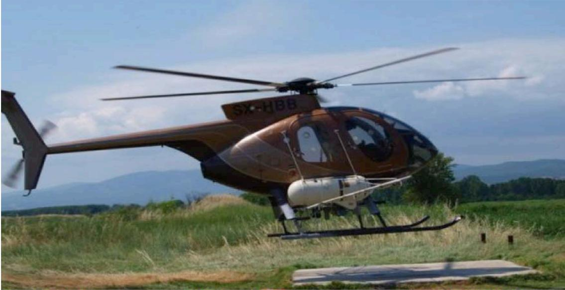
**Photo 4:** The helicopter fitted with the spraying apparatus
