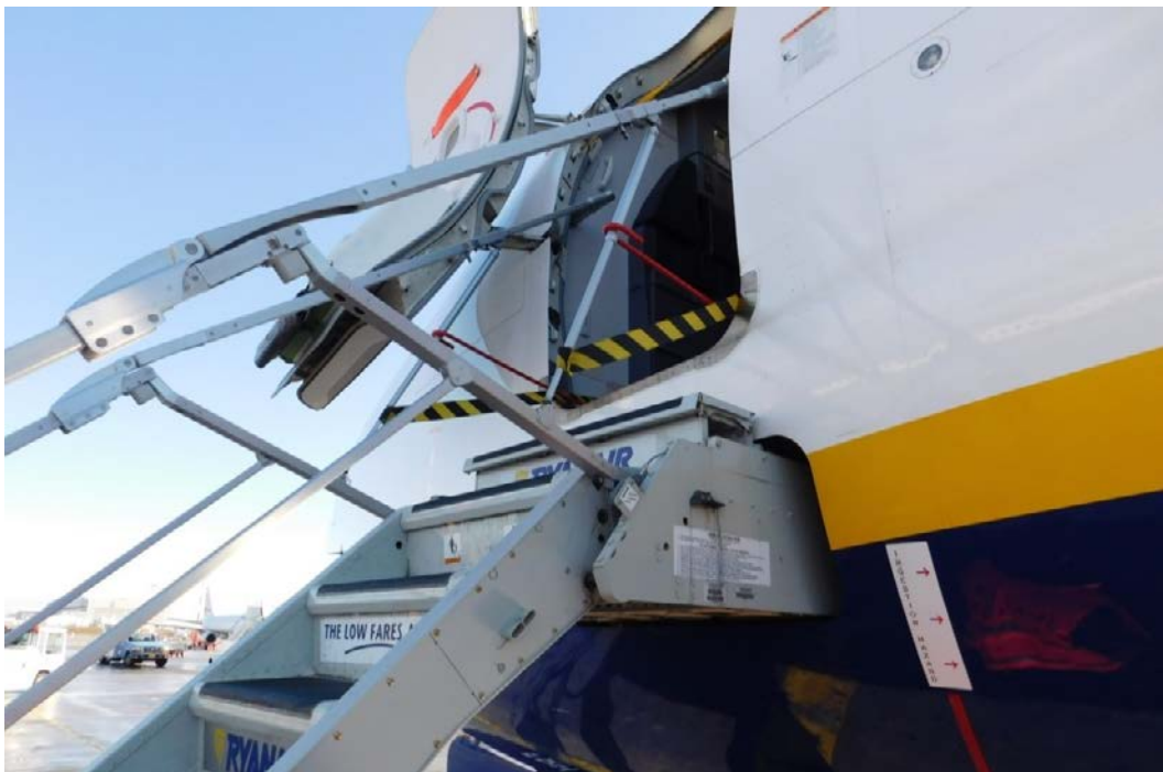
Photo 2: Uppermost part of the forward folding stair of the aircraft.
