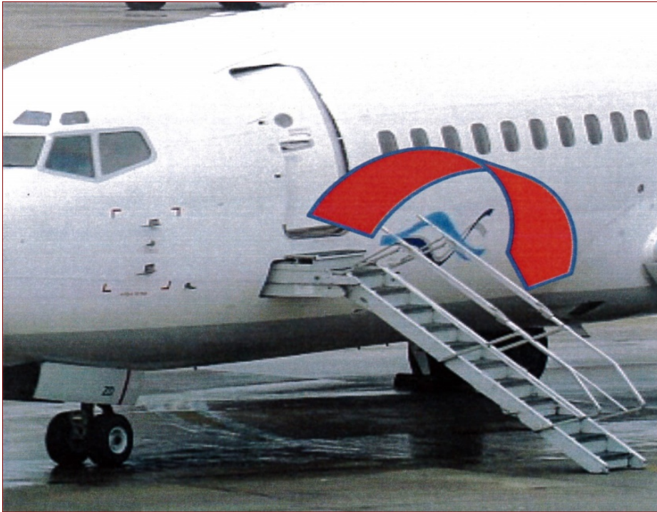
Photo 3: The direction of fall of the fuel personnel from the folding stair.
